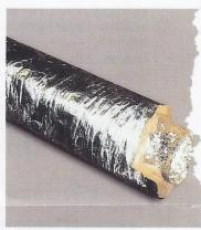
Construction features an inner duct wrapped in 25mm fibreglass insulation. An outer jacket, comprising wound multi-layer aluminium polyester laminated fabric reinforced with fibreglass yarn. The ducting is easy to connect to round or oval ducting and no special tools are required.
